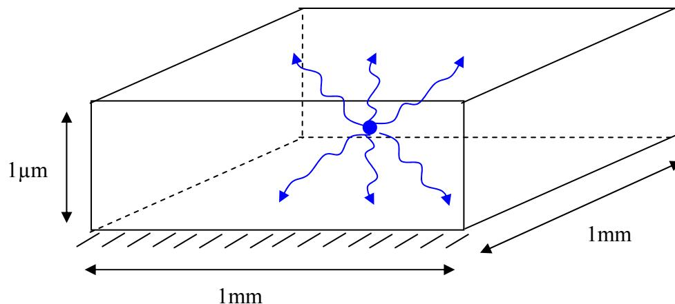
The dimensions of the LED are  $1\text{mm} \times 1\text{mm} \times 1\mu\text{m}$ . The light (in this simple model) is generated homogeneously in a point source in the middle of the LED. The LED is formed by a single crystal of GaN with the following physical properties:
